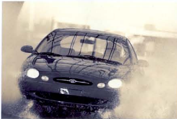
The 40 mph saltwater drive tests Taurus' ability to ward off corrosion.
